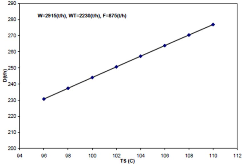
Figure 10. Effect of steam temperature on plant productivity
