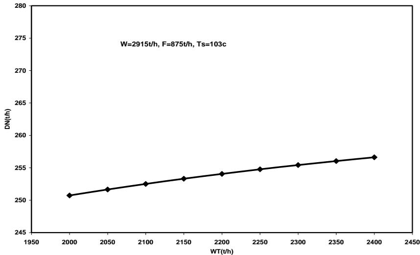
Figure 4. Effect of seawater flow rate on plant productivity
