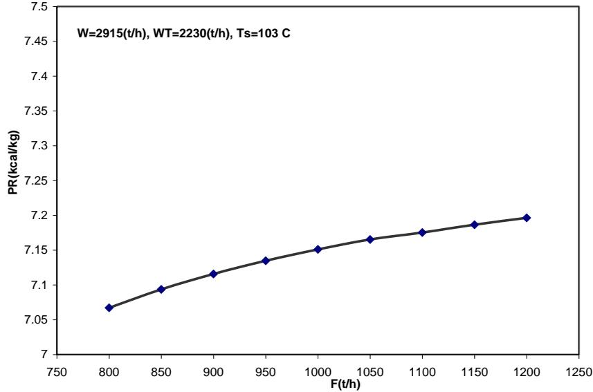
Figure 9. Effect of the make-up flow rate on performance ratio
