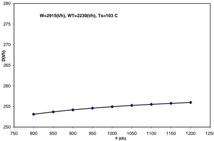
Figure 8. Effect of the make-up flowrate on plant productivity
