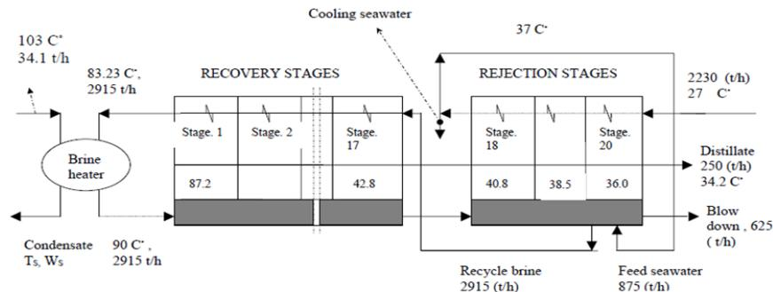
**Figure 2. Heat balance diagram for multistage flash desalination plant presented by the contractor**
