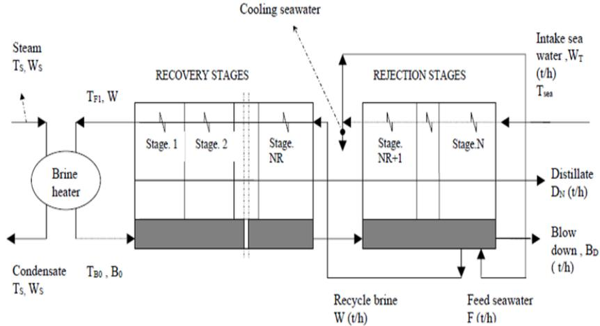
Figure 1. Recirculation brine multistage flash (MSF) desalination plant
