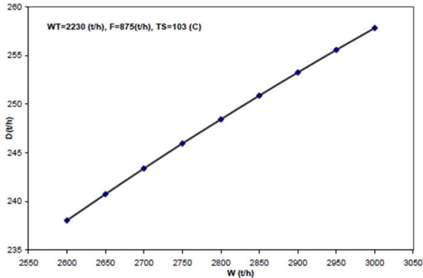
Figure 6. Effect of brine recirculation flow rate on plant productivity
