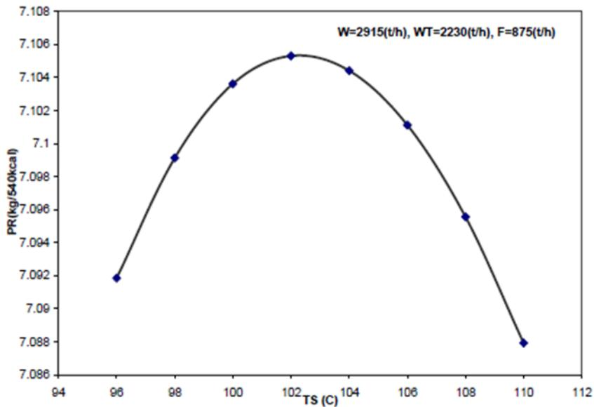
Figure 11. Effect of steam temperature on performance ratio
