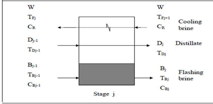
Figure 3. General stage in an MSF plant
