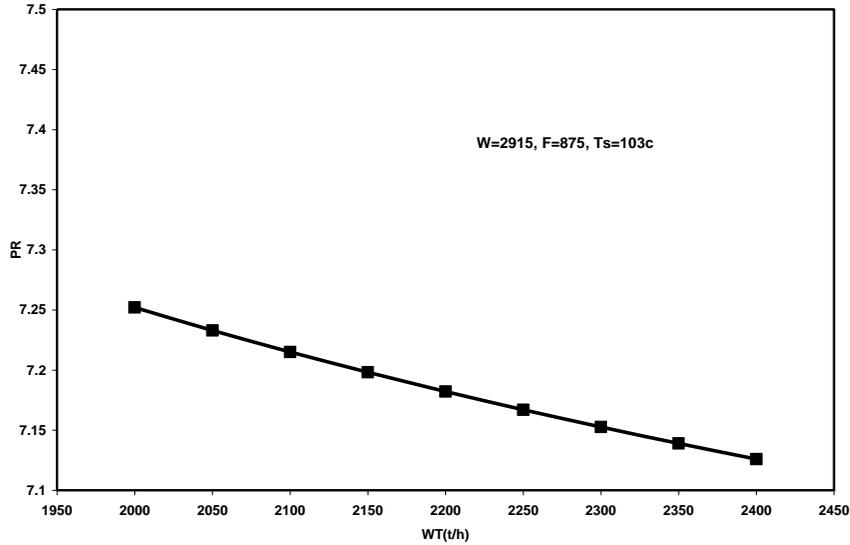
Figure 5. Effect of seawater flow rate on performance ratio
