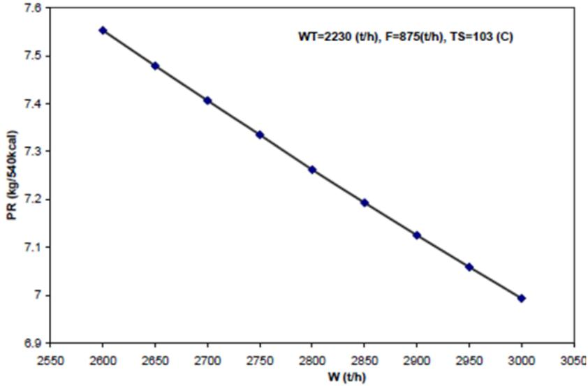
Figure 7. Effect of brine recirculation flow rate on performance ratio
